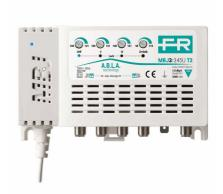
4-input (III+DAB, IV, V, UHF) multiband TV indoor amplifier with 20dB gain and up to 115dBμV output level on UHF band, separate amplification with independent level adjustment (20dB) for each input and low noise figure. T2 technology with UHF cut band for LTE 4G @790MHz and 5G @694MHz.
